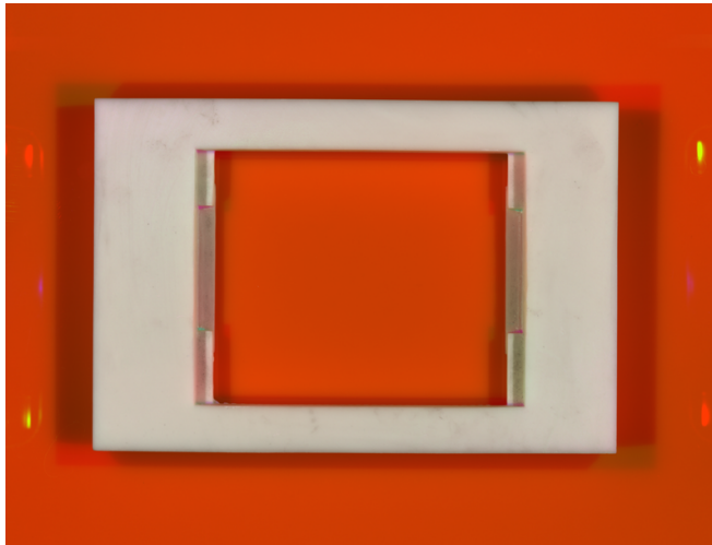
Stage, 3D-printed with white resin.
